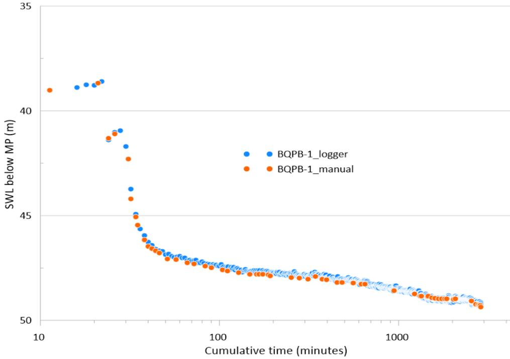
BQPB-1 Pumped Bore - Recovery vs. Log time
