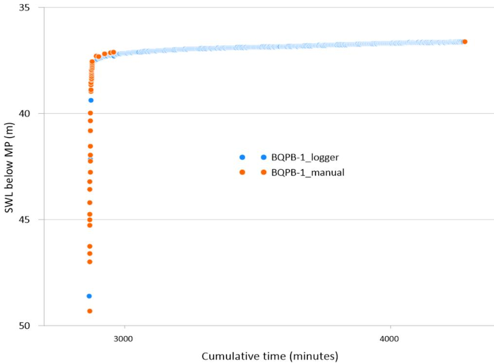
Monitoring Bores, BQN1 cluster - Pumping Test - Drawdown & Recovery vs. Log time
