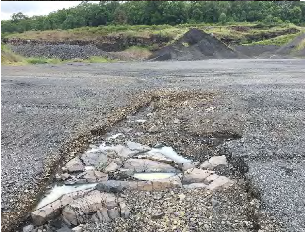
Plate 4 16/03/2017 Fractured basalt on Quarry floor near SW4.
