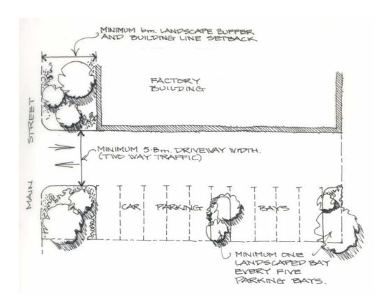
Internal roads and car parking areas shall be constructed of bitumen seal or similar material and are to be drained and marked to Council's satisfaction. Design details are to be submitted to Council for approval with the Development Application.
