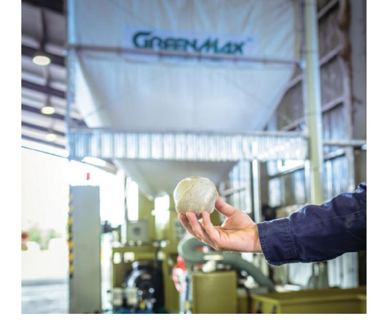
The new machine can process up to 300 kilograms of polystyrene per hour by crushing and sorting the foam which is then pushed through heating rings that melts and cuts the foam.
