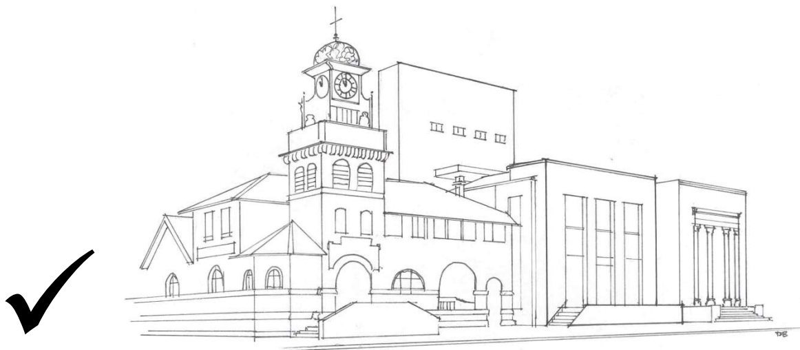
Figure A.9: Bulky buildings can be visually broken down into smaller components to better reflect the character of their neighbours. The bulk of the central building has been placed behind a smaller facade so it does not dominate the streetscape.
