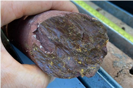
Image 1: "Slikenside" (Geotech term) – evidence of historic landslide at this location
