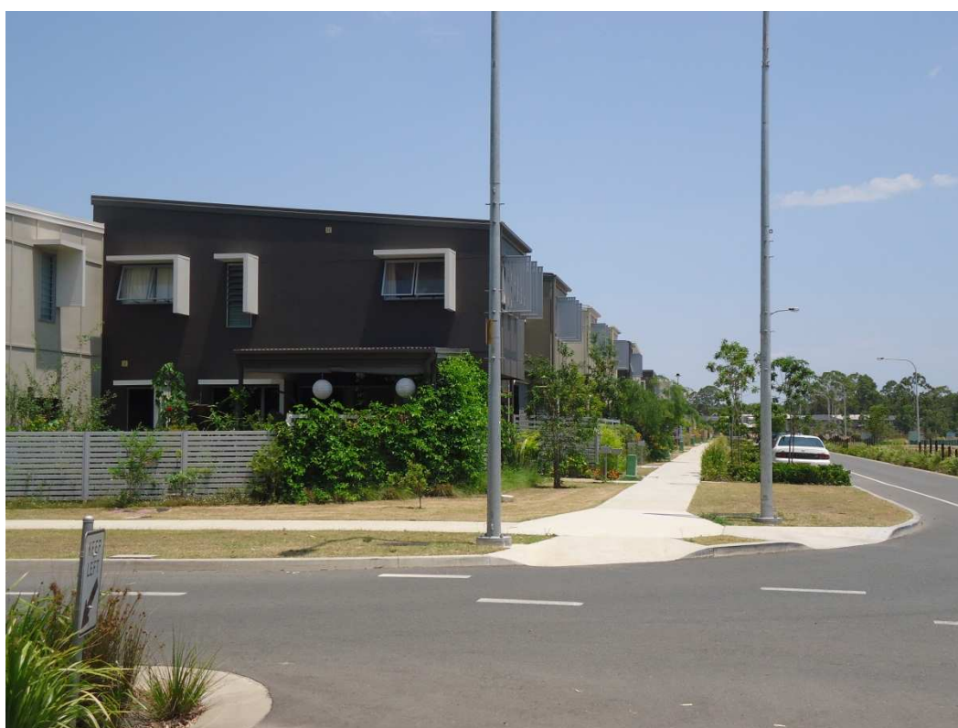
Figure 9: Dwellings on corner lots address both street frontages through the inclusion of modulating elements in the building elevation such as: recesses, projections, windows, awnings and sun-shading devices, to avoid blank walls on side elevations reducing the amenity and safety of the streetscape.
