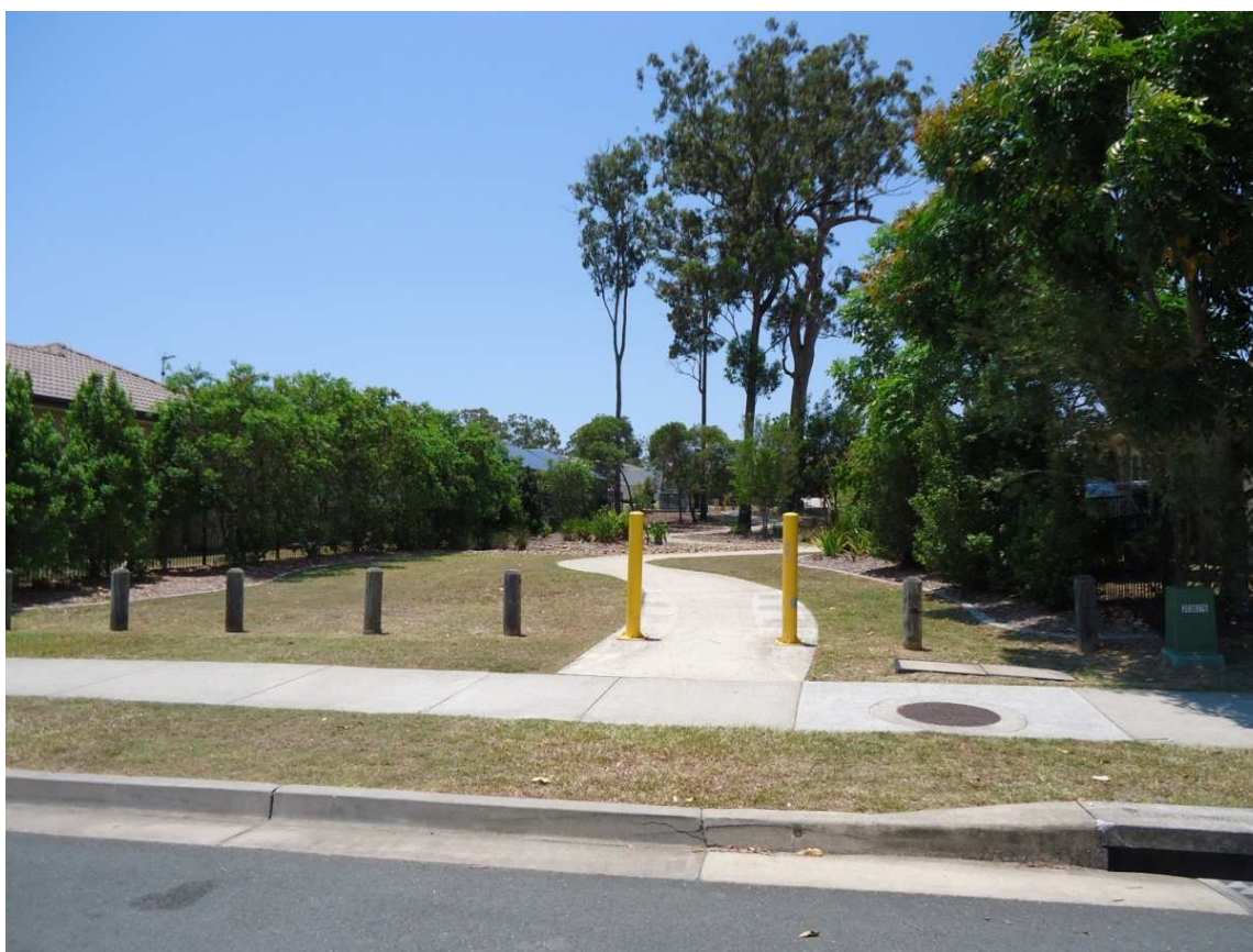
Figure 4: Easements and inter-lot linkages for public pathways are minimum 10 metres wide to allow space for amenity landscaping and lighting so that casual surveillance of paths is maintained. Pathways are well lit and designed for 24 hour use.
