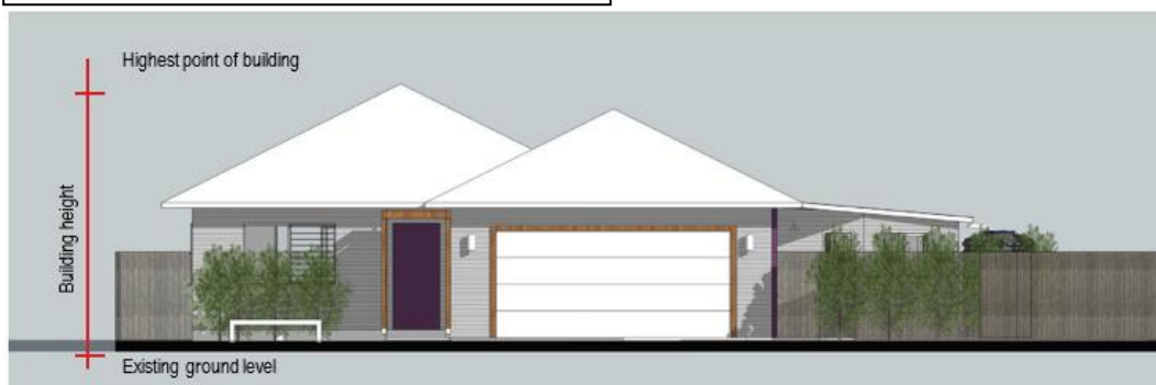
Figure 4: Measuring Building Height
