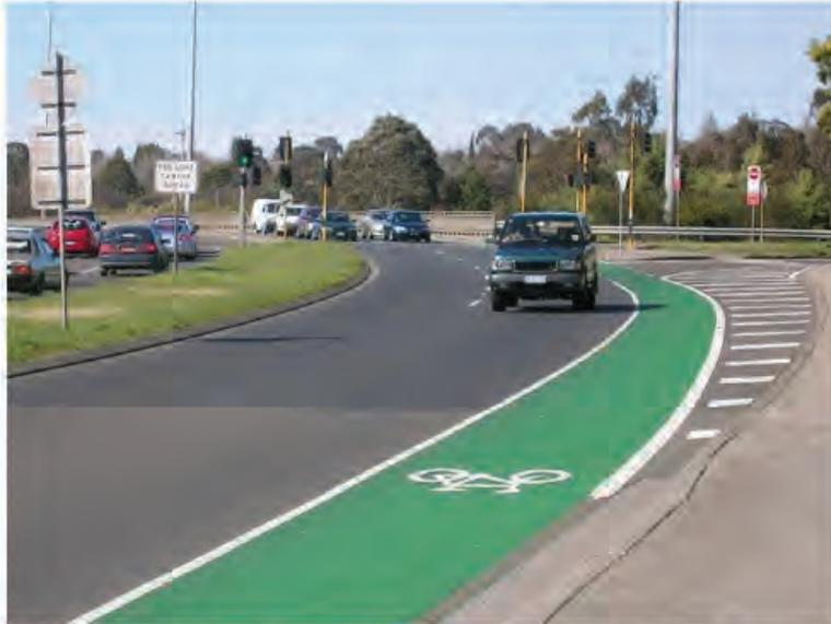
Note: Green coloured surface treatments should only be used to increase driver and cyclist awareness of a bicycle lane, and to discourage drivers from encroaching into a bicycle lane. The treatment should be used sparingly to maintain its effectiveness.
