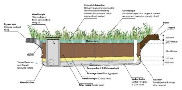
Illustration 1.1 **Typical cross section through a bioretention system (with under-drains)** Illustration courtesy of South East Queensland Healthy Waterways Partnership (Water by Design program)
